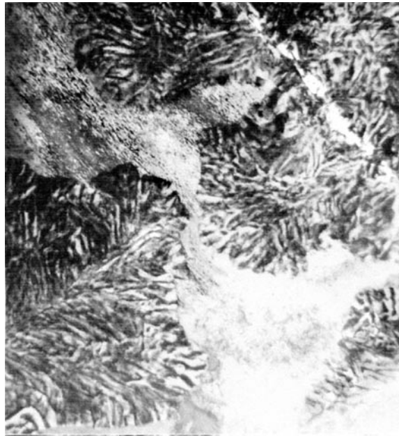
Figure 12. Near lamellar nodules exhibiting cube–cube branching with cube templating by the initiating modulation. Note that the two main dendrite cores to the right and left are aligned with the remnant modulations and their nucleate instabilities (figure 10). Lamellar spacing approximately 0.1 \mu\text{m} .
