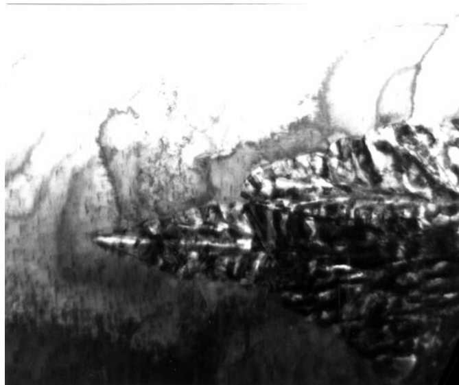
Figure 11. Directional [100] dendrite with bainite-like two-phase lamellar side-branches coarsened from the modulation instabilities of figure 10 evolving into the nodules of figures 12 and 8. See figure 2 for scale of modulations.
